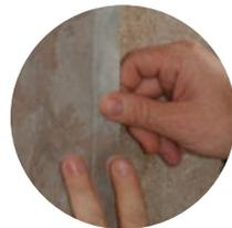
*FLEX* can be bent around corners after heating (from 40°C). In the approach *FLEX* is also 3D-formable.
