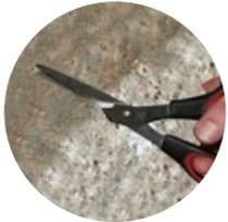
The material can be cut with scissors or a carpet knife.
